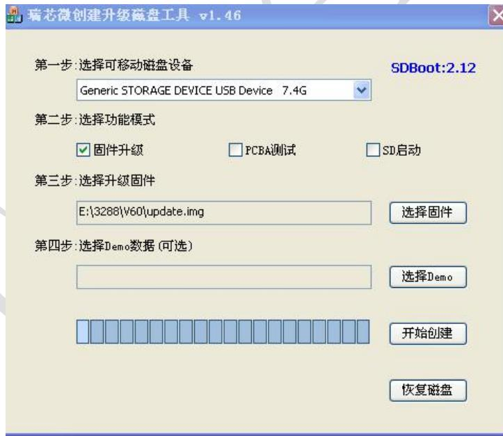
Step3, In function mode, check “**固件升级**” , “**选择升级固件**” ( which means zipped firmware update-android.img in Android)
