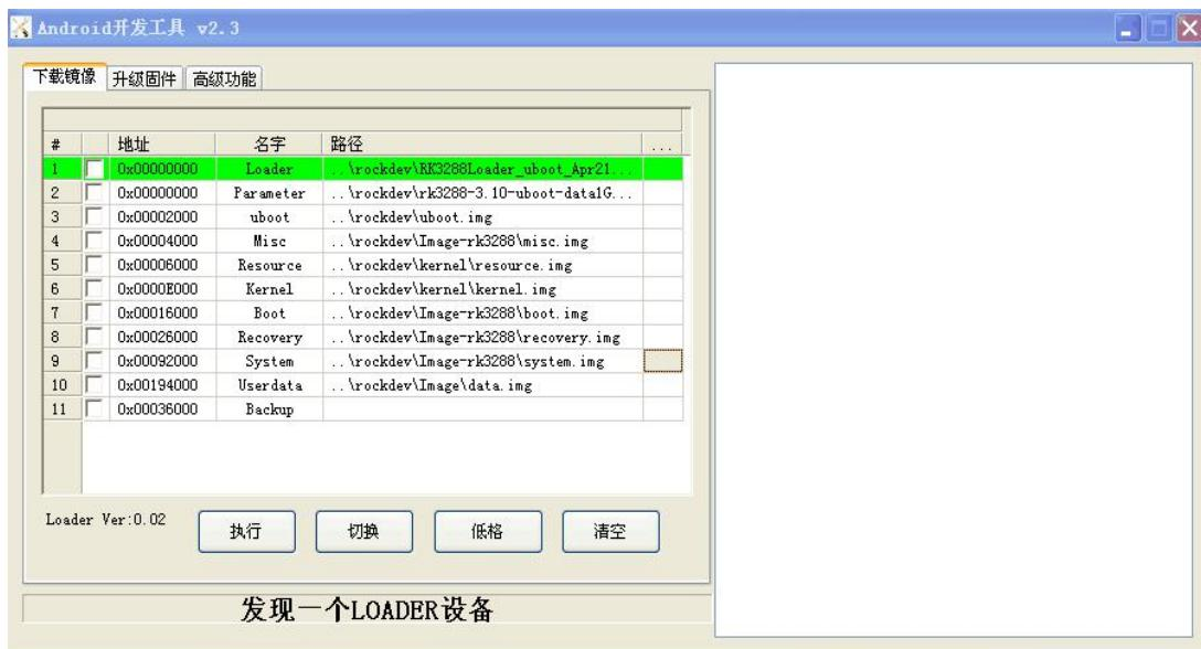
Or update unit firmware update\_linux.img: Check firmware update\_linux.img, and click '升级' (Upgrade) button.
