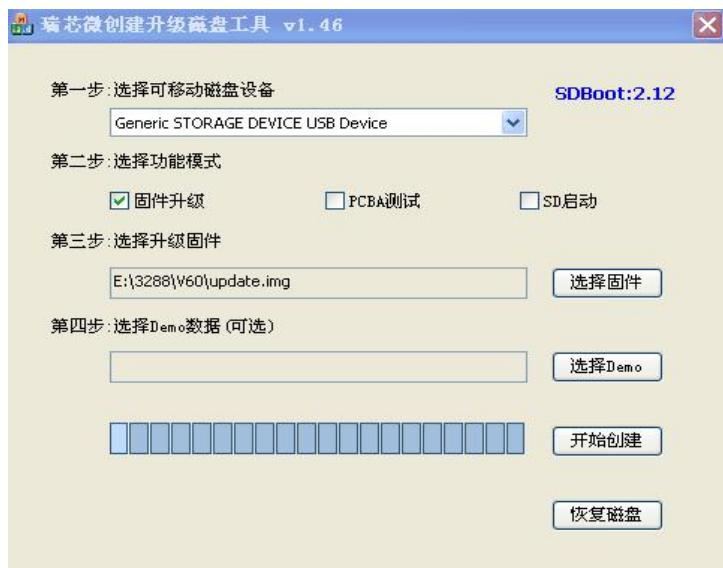
Step2, Insert TF into PC, and software tool will find TF card, like:
